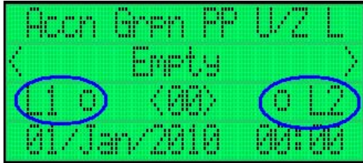
Figura 17a – led “apagado”.
